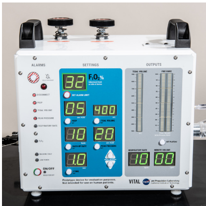
VITAL (Ventilator Intervention Technology Accessible Locally) is a new high-pressure ventilator developed by NASA and tailored to treat coronavirus (COVID-19) patients. Credit: NASA/JPL-Caltech
