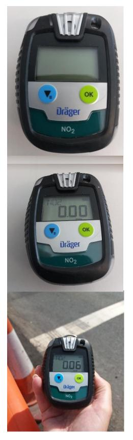
To switch **on** press the OK button and keep your finger on the button for 3 seconds. (You will see the seconds counting down on the reader).
