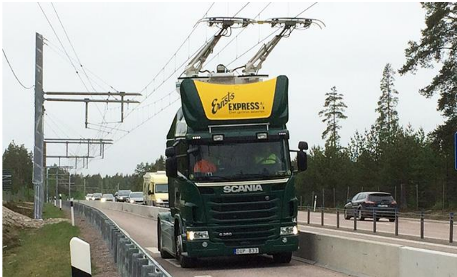
Figure: 6.9 OWPT trial on E16 highway in Sandviken 159
